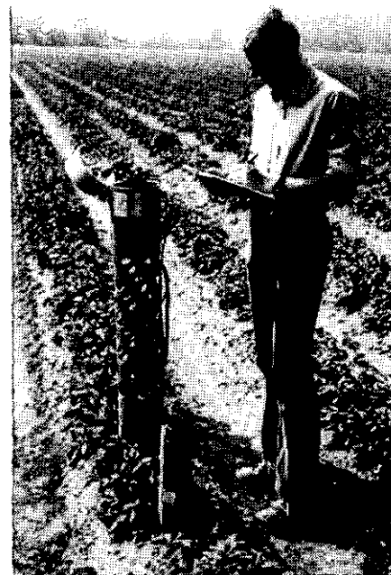
An Irrigation Management Consultant measures soil water in the field using a neutron probe .
