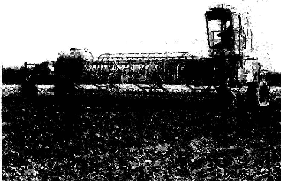
An experimental tillage and crop treatment gantry at AFRC Engineering.
