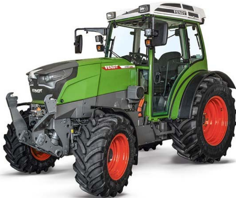
Fendt e100 vario electric tractor 100 kWh battery – V2G ready on sale 2018 in Germany
