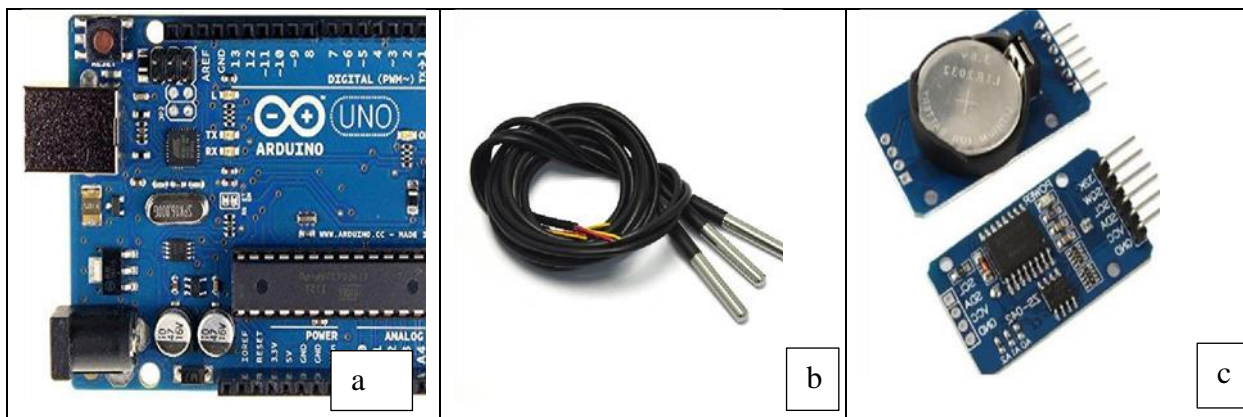
Figure 3: Arduino components for programming (a) Arduino board;(b) digital temperature probe; (c) real time clock
