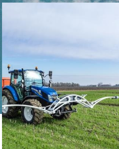
CropXplorer sensor for optimized N-balance
