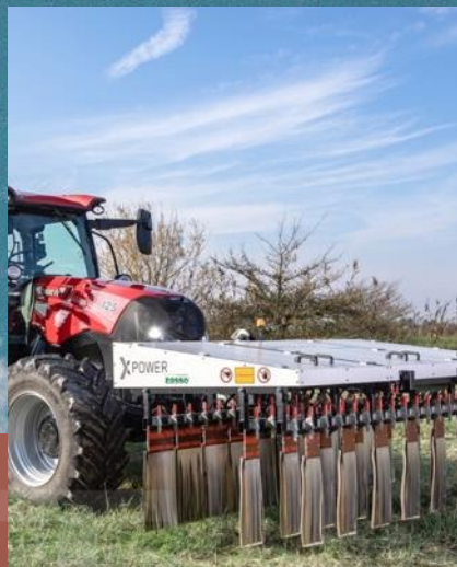
XPower electro-herbicide for zero-chemical weed control
