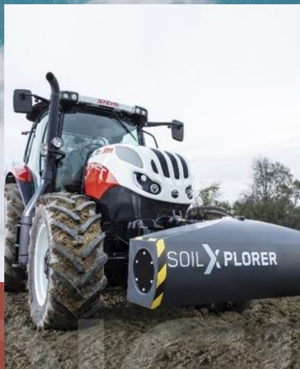
SoilXplorer with the real-time soil scanning system
