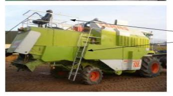
Handrails fitted around areas at height and access steps, note position of fire extinguisher
