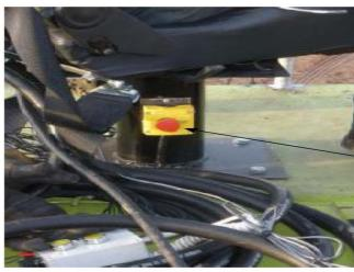
Emergency stop position below seat of flame thrower operator
