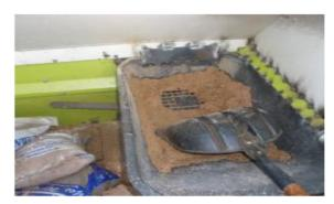
Grit introducing hopper, note moving parts below mesh, do not remove mesh.
