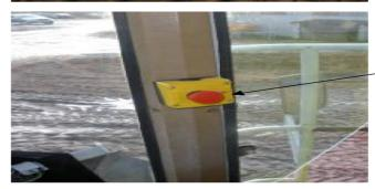
Emergency stop fitted in cab of machine for driver too operate.
