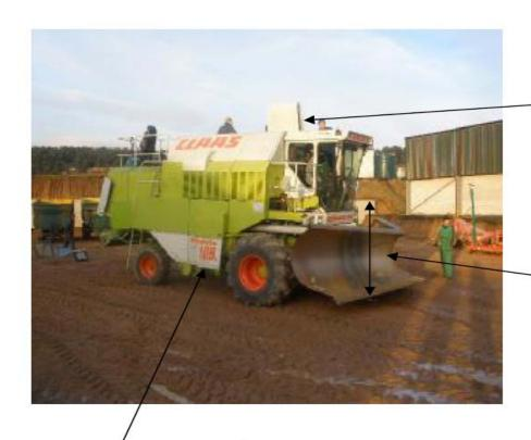
Note engine cover in up position, moving engine parts such as fan blades and fan belts located below this hatch, hatch should be closed when running vehicle
