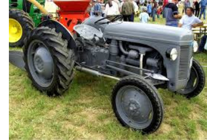
Massey Ferguson T 20 Tractor 15 Kilowatt, safe load 3 tons. Can work a 2 furrow plough.
