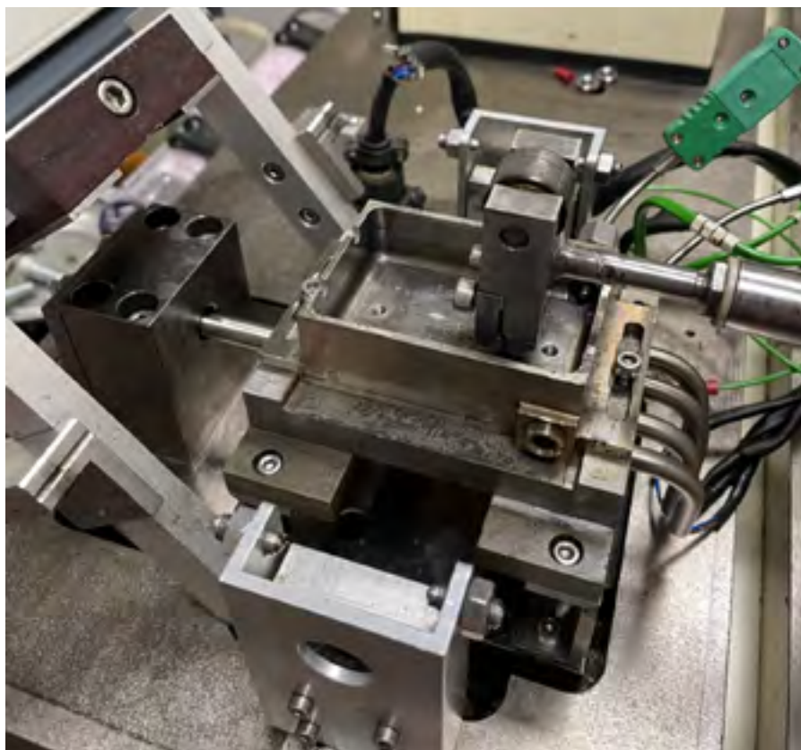
Phoenix Tribology TE 77 – the apparatus used for many reciprocating lubricated tests
