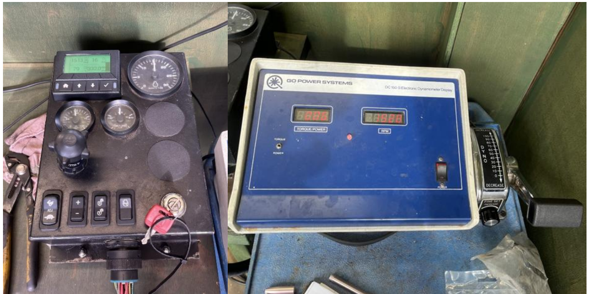
Figure 25 John Deere Controller and Go Power Systems DC 150-s Electronic Dynamometer Display
