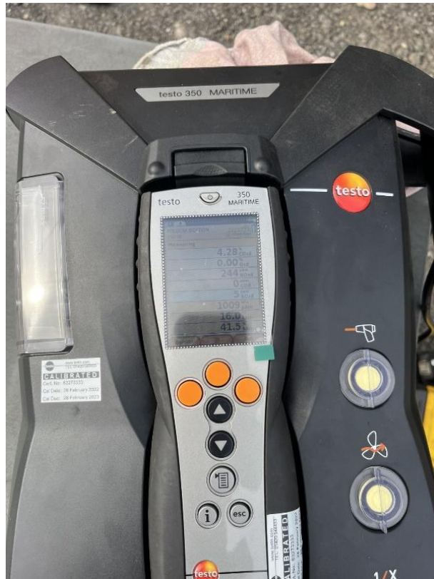
Figure 26 John Deere 4045HFC09 Testo 350 First Emissions Reading at 100% Load
