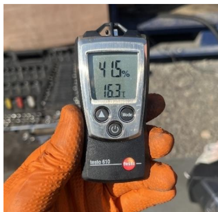
Figure 24 Testo 610 Used to Measure Air Temperature (°C) and Humidity (%)
