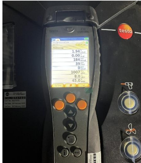
Figure 23 John Deere 4045HF158 Testo 350 First Emissions Reading at 100% Load
