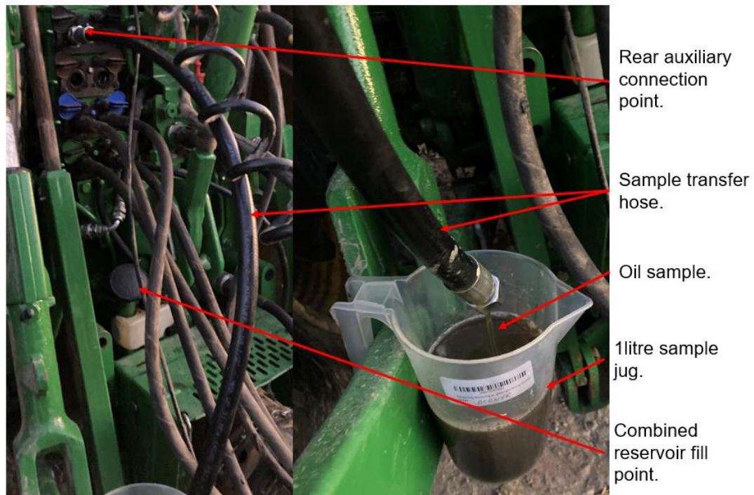
Figure 8. Transmission oil sample procedure Fendt Tractors.
