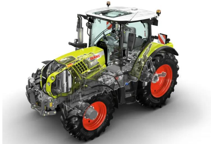
Figure 7: A render of a CLAAS ARION 630 showing its internal powertrain and driveline [36].
