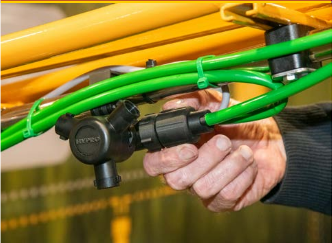
Knights Smart-Inject system injects neat or semi-dilute plant protection products for precision spraying
