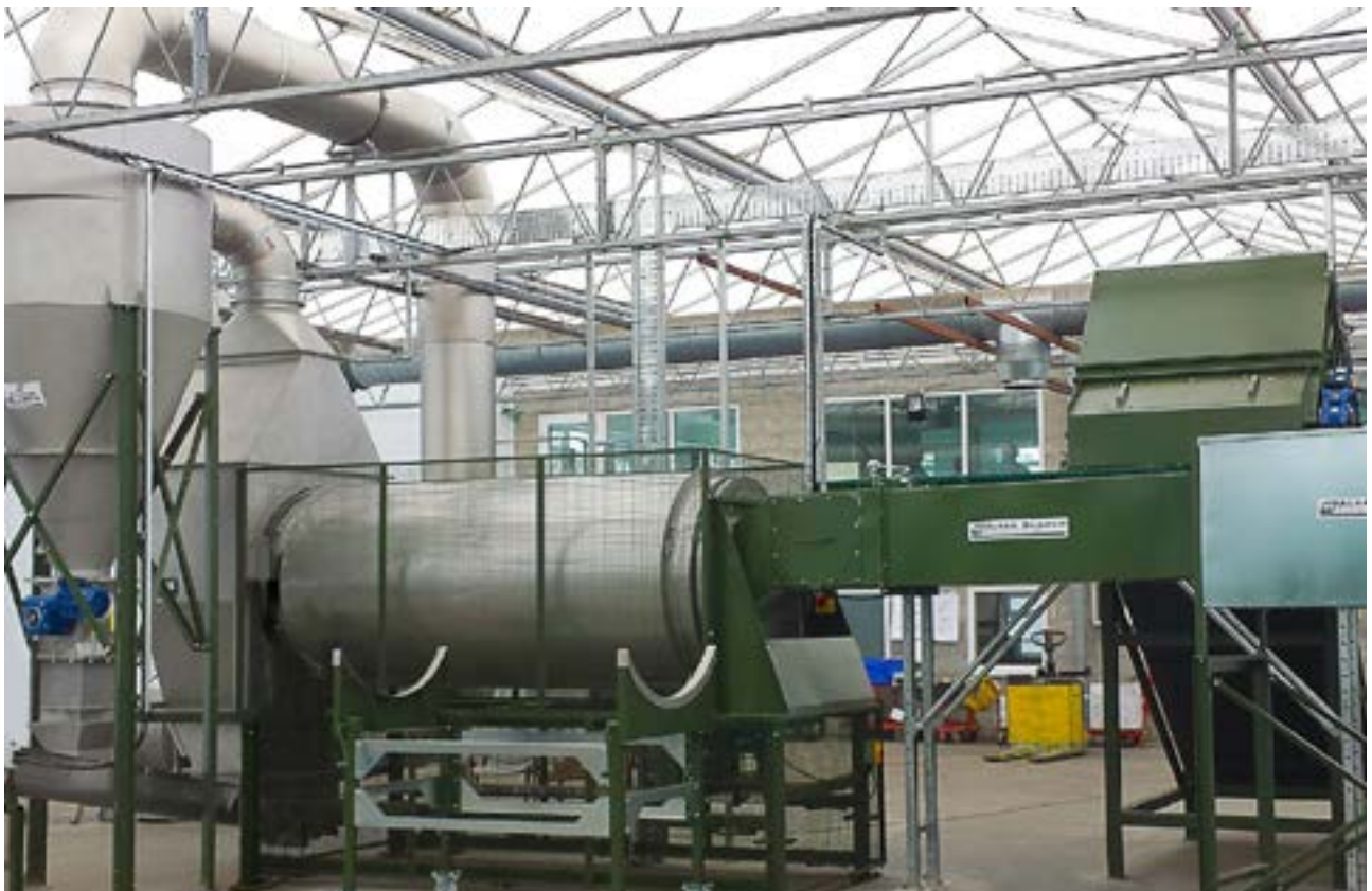
Medical cannabis installation incorporating rotary driers, stainless steel drum, dust collection and heating furnace
