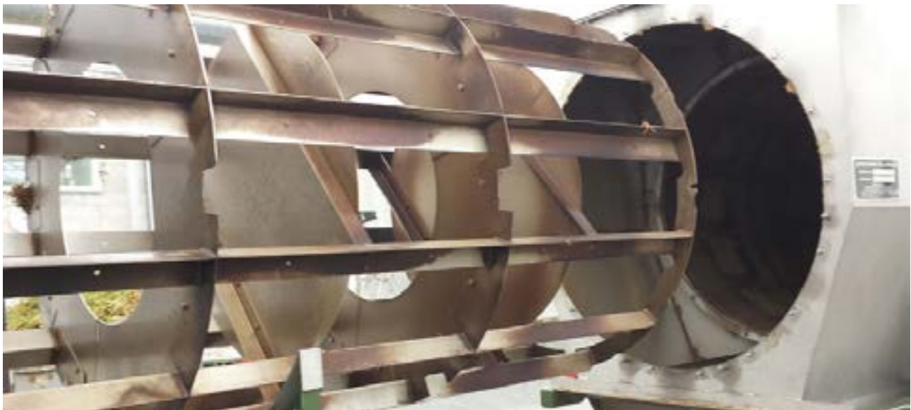
Insert cartridge with lifting paddles being fitted to the drying drum of a cannabis drier.
