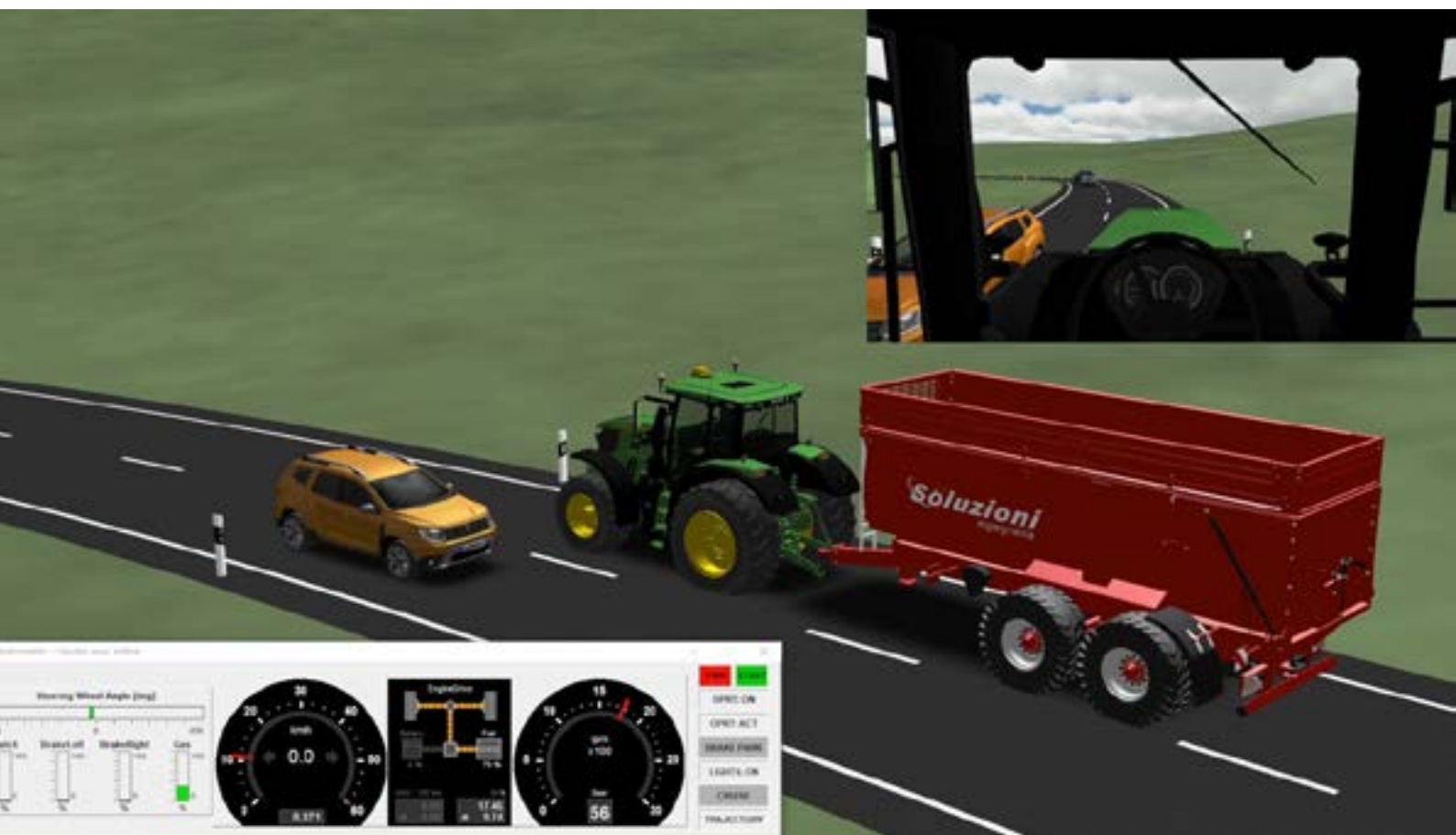
This image depicts a tractor simulation towing a trailer on a road with oncoming traffic. The inset picture illustrates the simulated driver's perspective, showing a passing car and an approaching lorry. The display panel indicates the operating conditions of the simulation: the tractor is moving at 10 km/h, the engine is running at 1,500 rpm, the steering wheel angle is 10 degrees, and the throttle position is at 10%.
