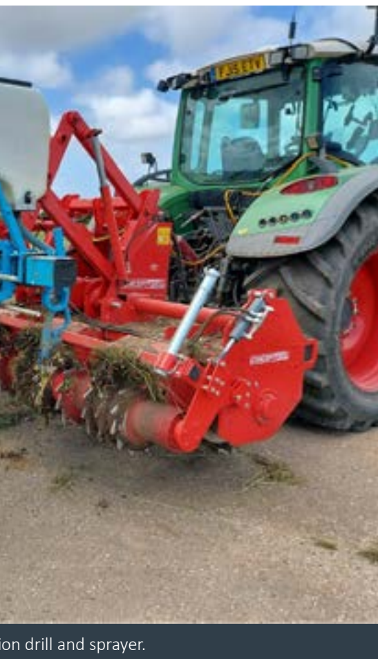
...d crimper roller to mulch standing vegetation...
