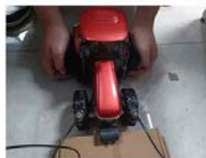
fig 7 - Example of the model prototype tractor (1:18 ratio) fitted with sensors on the front wheels to measure vibrational characteristics with shocks (small drops) that are affected by tractor tyre stiffness and damping characteristics. Bottom Right - An example of the free vibration signal obtained after dropping the tractor system during one of the tests
