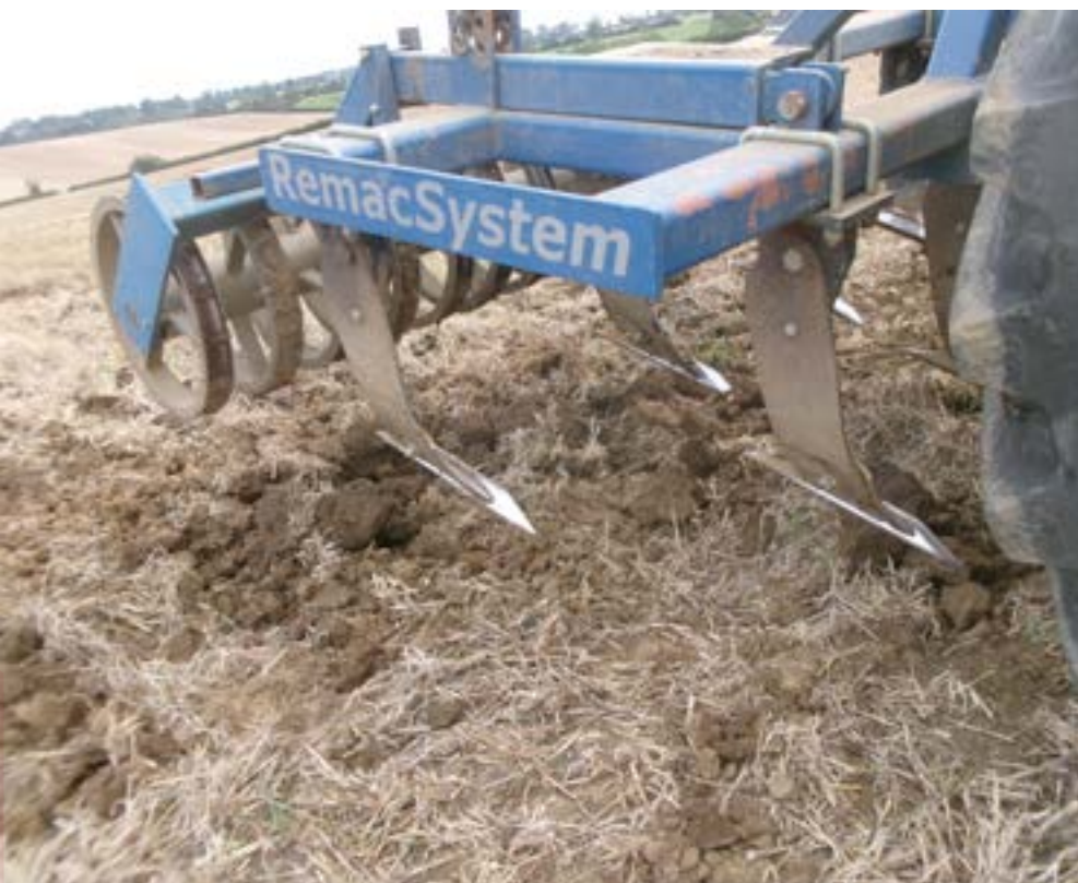
The host farmers cultivator uses angled tines to loosen soil but not invert it followed by press roller to give a reasonably level field.
