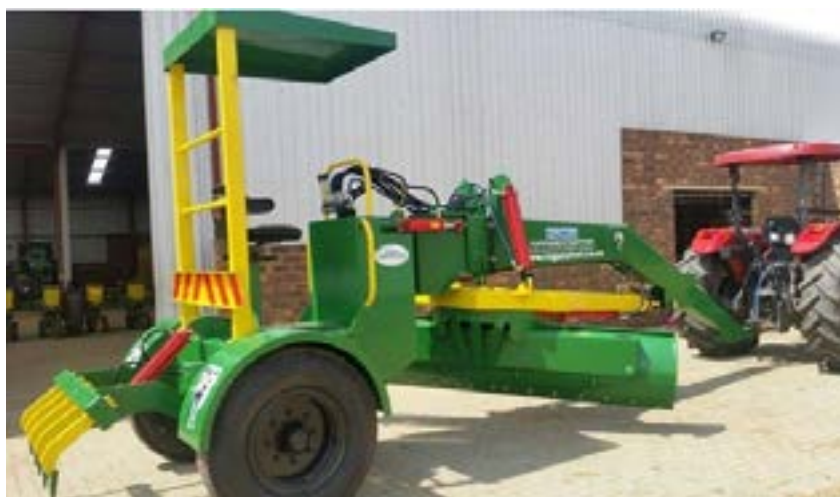
Fig 1 - 5 Tonne heavy towed grader and 75kW agricultural tractor, suitable for heavy and light grading.
