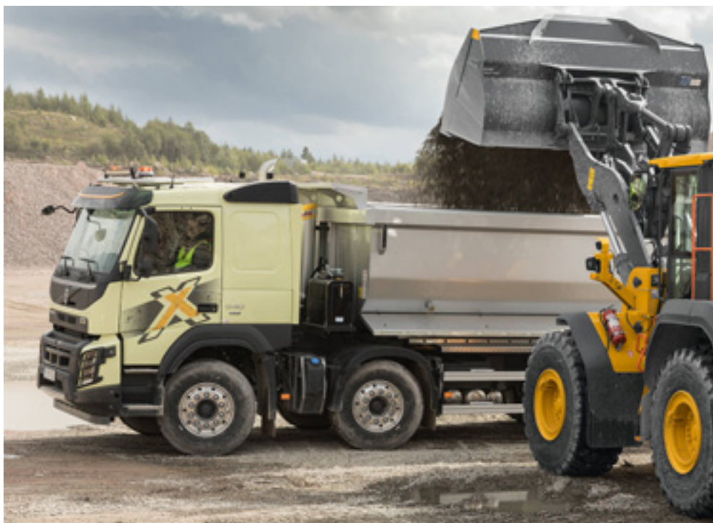
Volvo's electric conversion of a wheel loader has the same performance as its diesel counterpart
