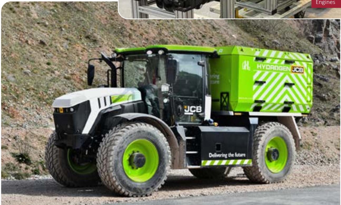
The mobile refueller stores hydrogen at 500 Bar
