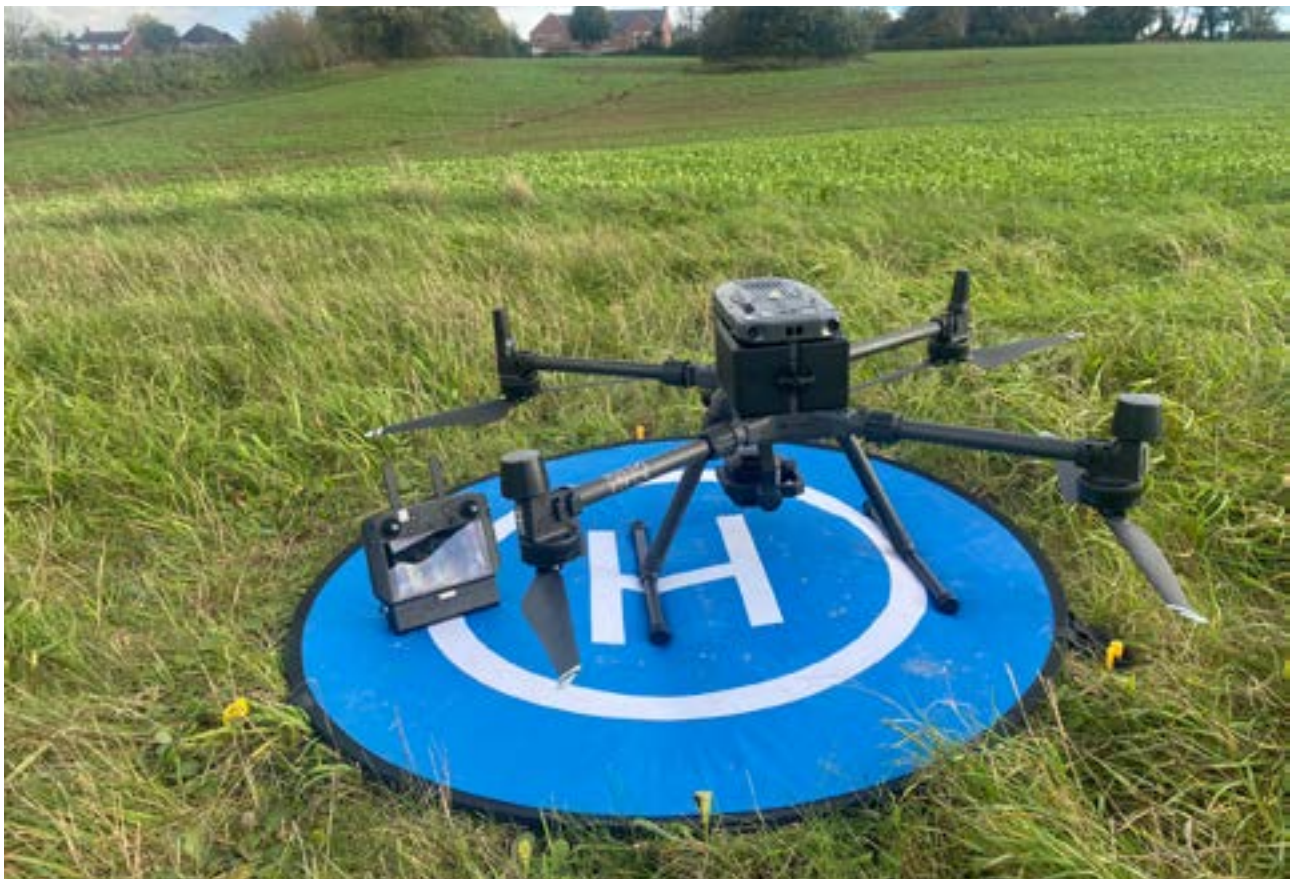
DJI Matrice 300 RTK drone used to obtain high resolution aerial photographs to create Digital Elevation Models (DEMs) and Orthophotomosaics for Josie's PhD research.
