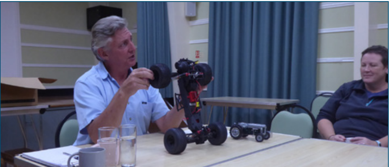
This model has independent suspension on all four wheels. However, when one wheel is raised there is a big weight transfer to the diagonally opposite wheel.
