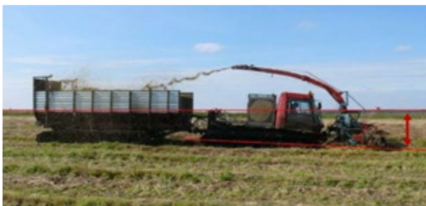
Cutting activities unbalanced by front mounted equipment
