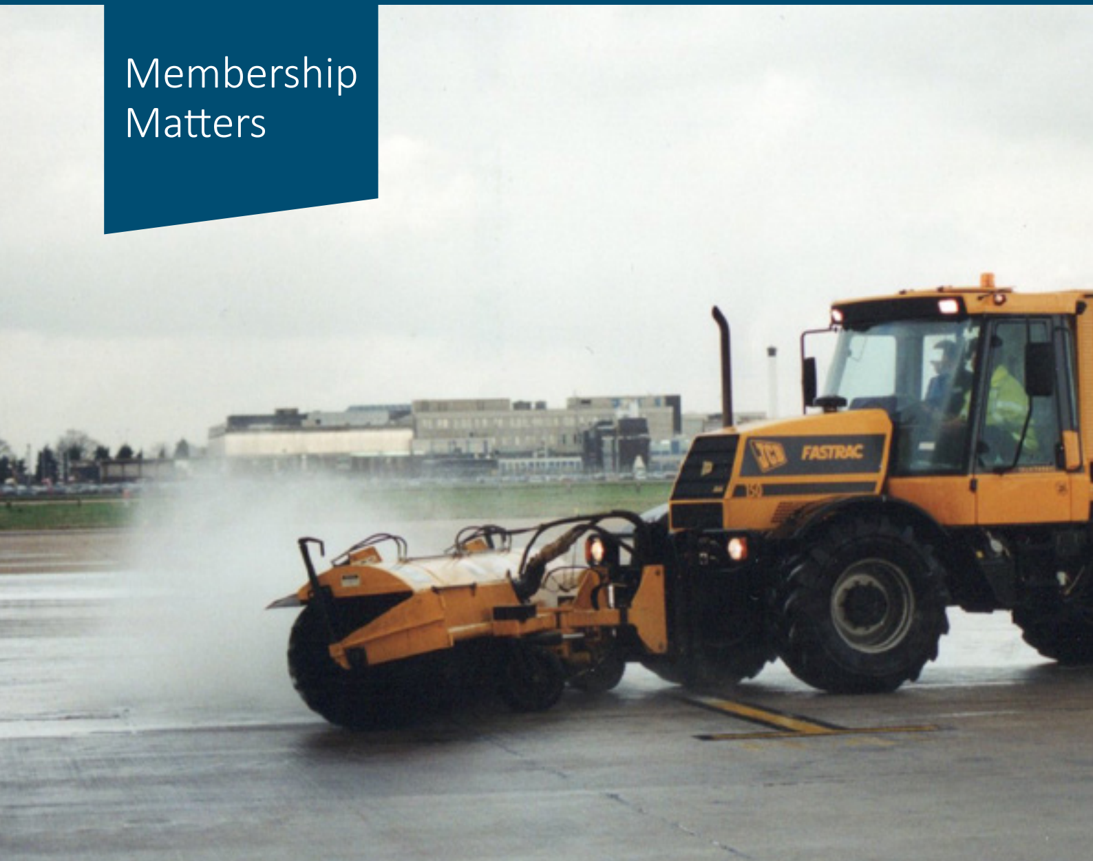
A purpose built unit for runway clearing built on a Fastrac at Heathrow
