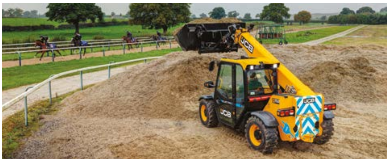
The 525-60E uses two electric motors, one for the driveline and the second to power the hydraulic system
