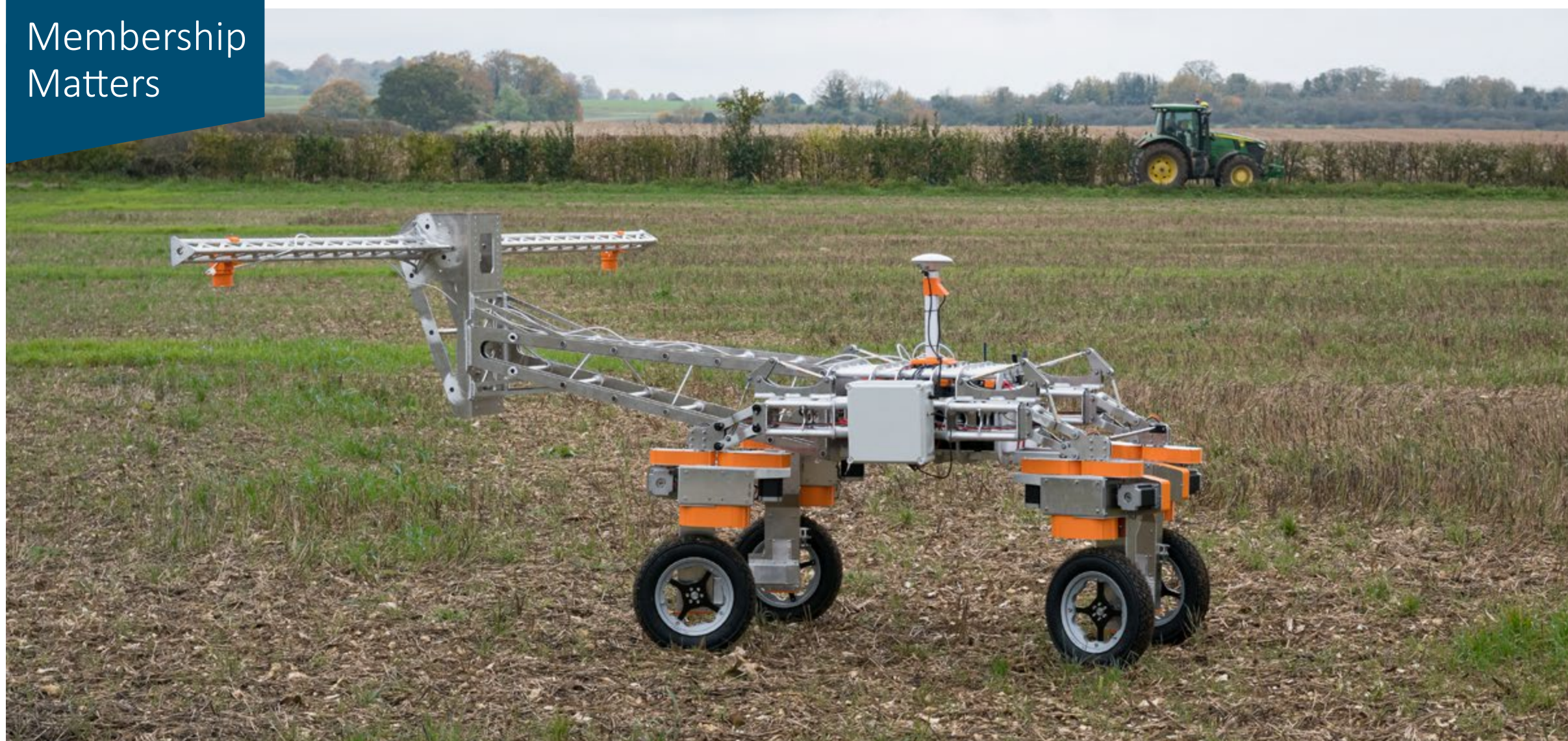
The next generation Tom design incorporates factors such as weather-proofing, speed, camera capacity and extended battery life.
