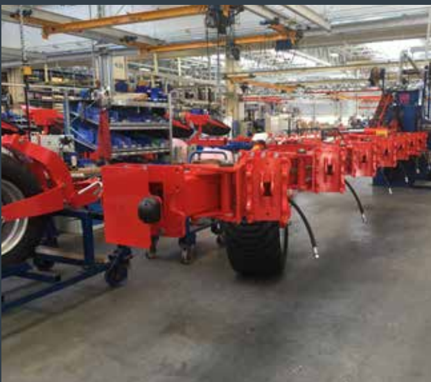
Here a 7-furrow reversible auto reset servo plough is on the assembly jig awaiting legs and mouldboards.
