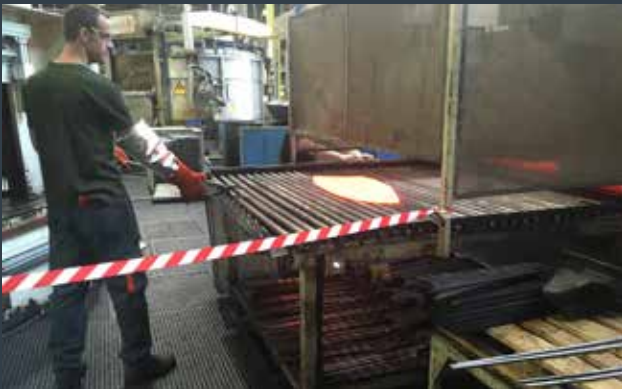
Next the mouldboards are heated in a furnace to approx 9200C for over 30 minutes.
