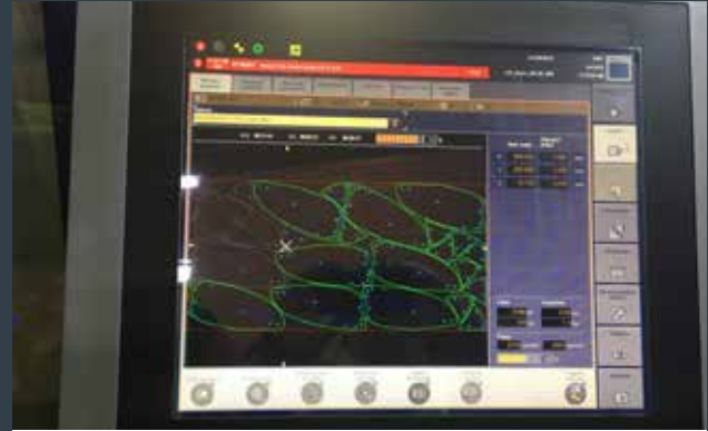
The laser cutter works out the best arrangement for the mouldboards on screen prior to cutting.
