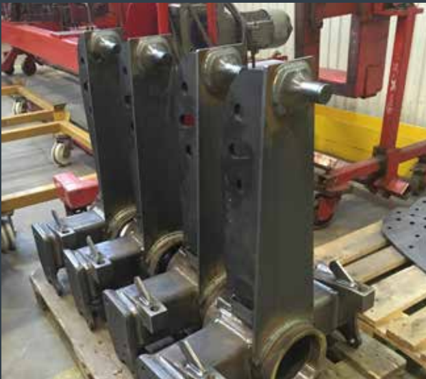
In a separate area the headstocks are cut and welded, prior to painting.
