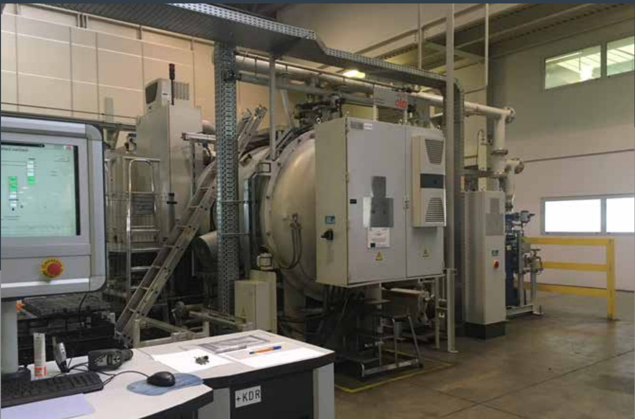
Since 2013, Vodnany has been the first plough factory in the world to use the ALD Vacuum Technologies GmbH high temperature, low pressure carburizing system. The mouldboards are heated to 1050 °C for 9 hours to open the steel structure and allow the carbon to enter this structure to a depth of 2.2-2.4mm. These mouldboards have a hard and resistant surface whilst still maintaining a ductile and flexible core.
