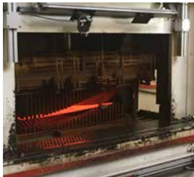
The pressing process - From the furnace they are pressed into the final shape.
