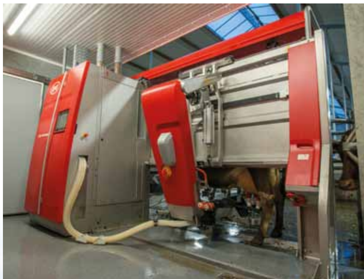
Lely Astronaut Automated milking machine
