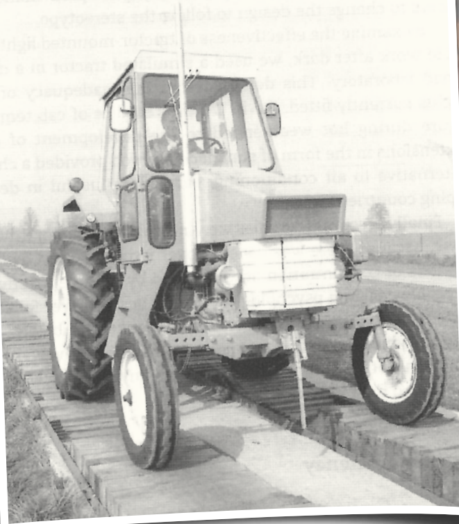
Suspended Cab testing
