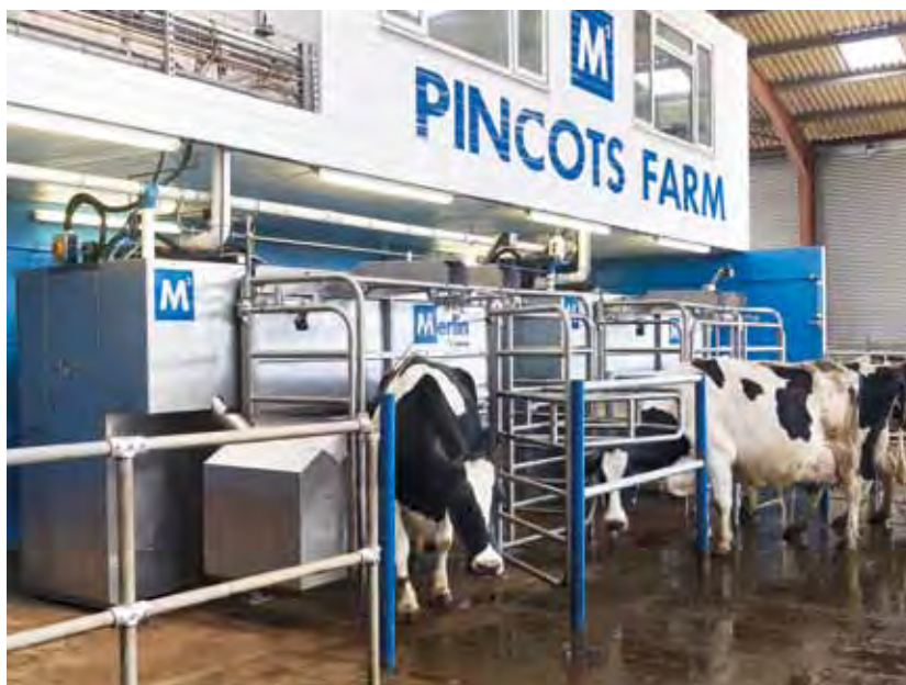
(ABOVE) Cows are encouraged into the automated milking stall by a feeding trough at one end. The rear gate closes when the animal's presence is detected by a photocell, which also records the cow's identity via an electronic tag © Fullwood
