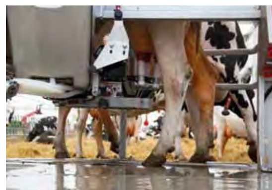
(ABOVE) A robotic arm in the milking stall uses stored coordinates to locate the position of the cow's teats, which are then washed by soft brushes on the arm. A laser tracking system is then also employed to improve more accurate positioning of the suction cups © Fullwood
