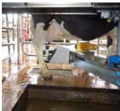
(ABOVE) A liquid flow sensor in the system that is electrochemically activated by milk can tell whether the cup is attached incorrectly and when the milk production has ceased, automatically allowing the suction cups to be removed. Inbuilt instrumentation can also run checks on the milk's quality and quantity © Royal Association of British Dairy Farmers
