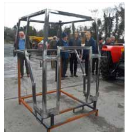
LEFT: William Ganly with IAGrE group RIGHT: Cab structure for TAFE tractor
