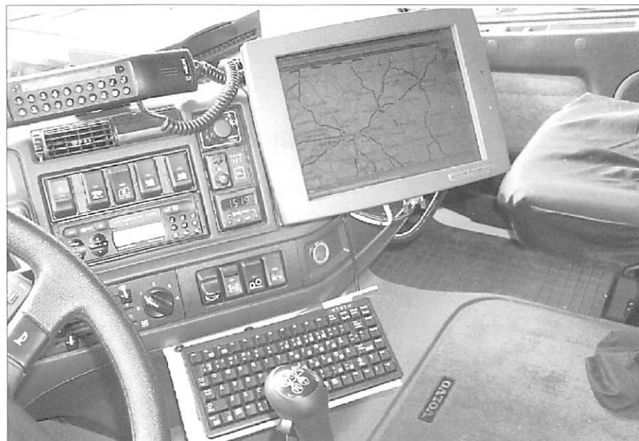
Driver's cab equipped with a computer and data transfer system.
