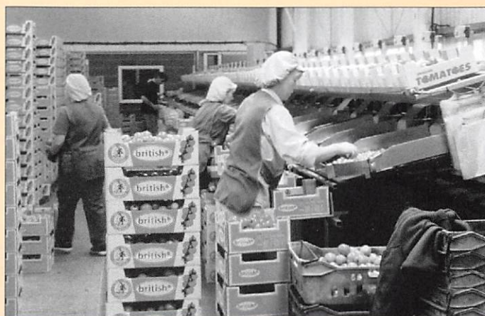
The manual input to an otherwise fully automated tomato grading line
