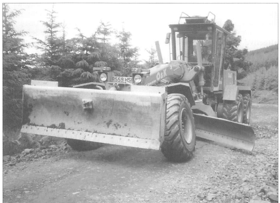
Fig. 7 Typical equipment for forest road maintenance
