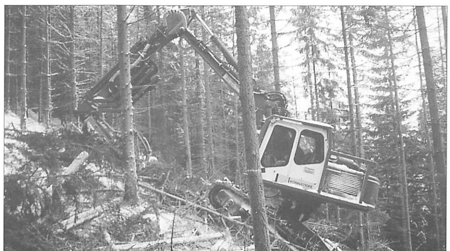
Fig. 2 The Königstiger tracked harvester operating on steep terrain.
