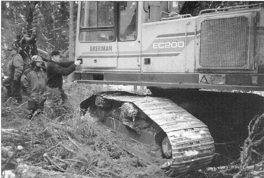
Bad machine parking, difficult access, footplate above recommended 0.4 m height, track grousers worn with little grip for the feet, and operator had to swing on the door and handle to assist in entering the cab
