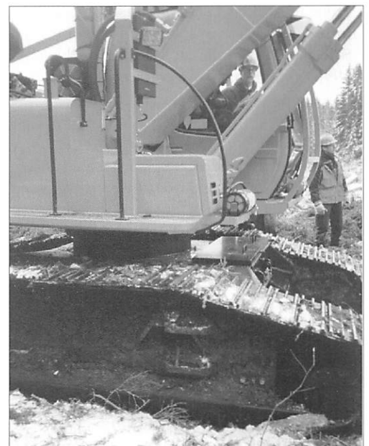
Good foot grips on track sides, well proportioned hand rails and grips, and footplates covered in anti-slip material
