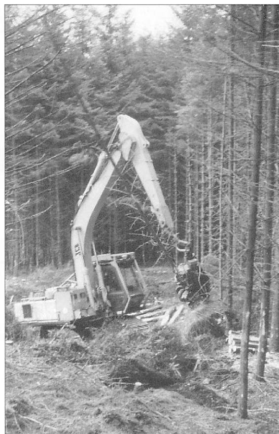
Poor posture and increased body tension continually coping with rotation of a cab tilted on a cross slope
