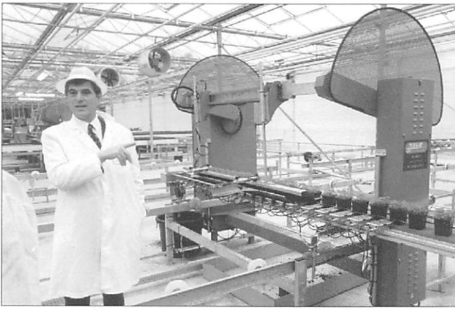
Tony Girard (Operations and Development Director for Hazlewood - VHB) describes the almost fully automatic system for filling and seeding the pot grown herb production. Shown also is the machine for lifting a row of pots to place them out on a flat.
