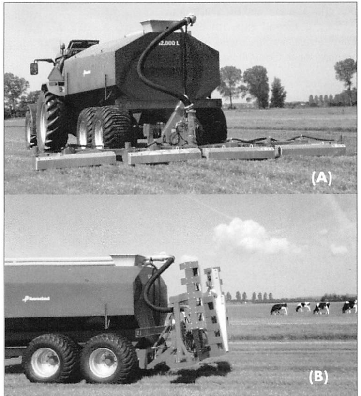
Fig. 4 DGI® mounted on a tanker. Working width is 6 m. The machine: (a) when running in the field; and (b) when it is folded for transport.
