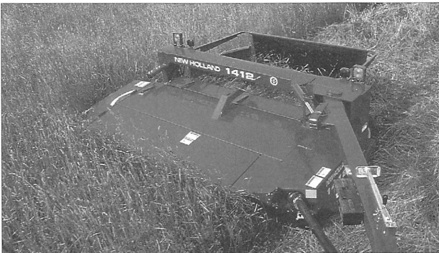
The new Model 1412 New Holland Discbine® features 2-speed flail conditioning to allow gentler conditioning for leafy legumes or more vigorous treatment for grass type crops for even more rapid curing. The 8-disc modular cutterbar has a 3 m cutting width. Swath width is easily varied from one to two metres without tools.
