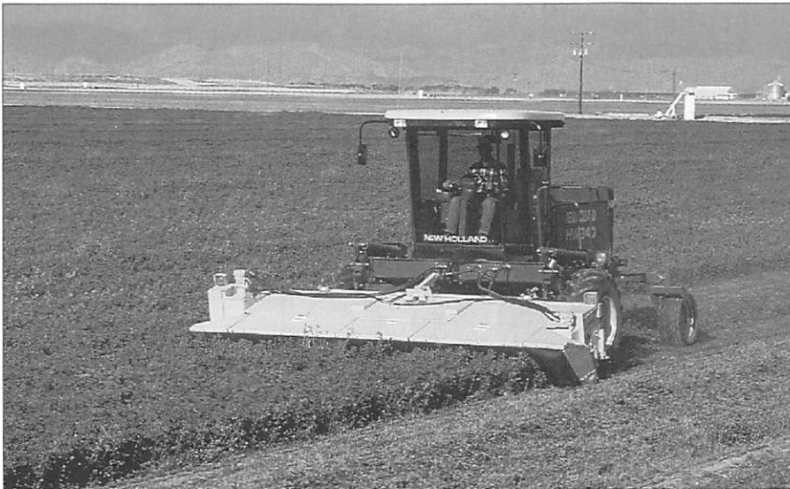
New Holland Model HW340 self-propelled disc mower-conditioners have 12 disc modules for a 5 metre cut. A 121 kW GENESIS™ engine provides ample power for all crops. A sicklebar header can be substituted for the disc-type cutterbar and draper headers with up to a 10 metre cutting width can also be adapted.
