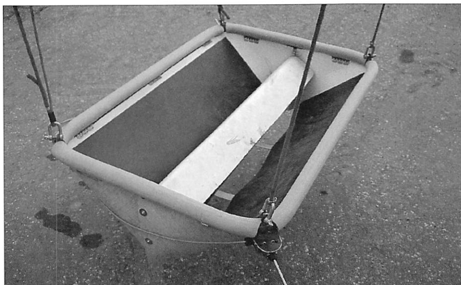
Fig. 4 SAC fall breaker attachment for harvester delivery conveyors.
