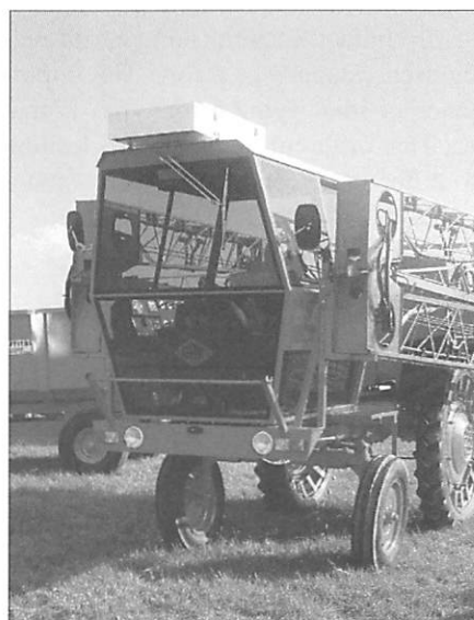
Fig. 2 Lateral stability limits operation of high clearance vehicles, such as self-propelled crop protection equipment.
