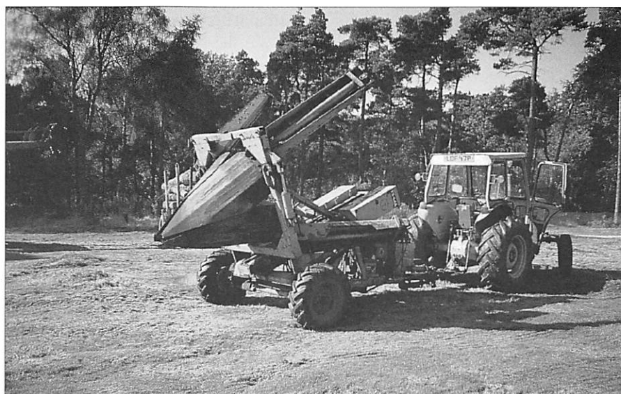
Fig. 1 The hazard of non-standard loads carried by tree transplanters.
