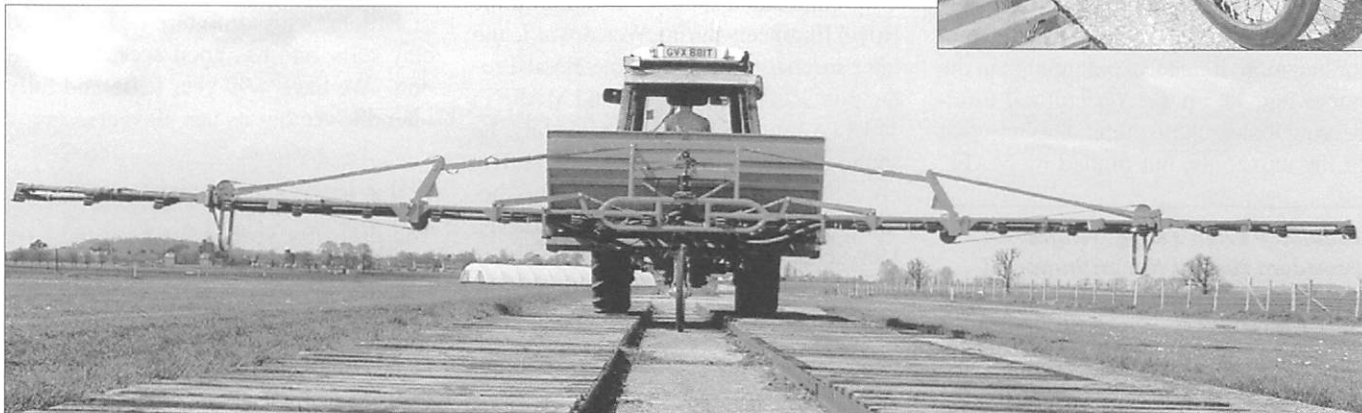
The twin-link boom suspension system developed at SRI on a fertiliser spreader. Inset shows the suspension instrumented for performance evaluation.
