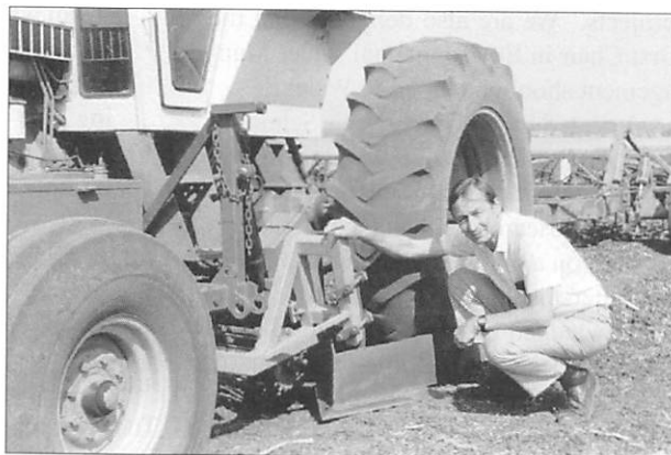
The author, with a tractor modified for controlled traffic (3 m track width).
