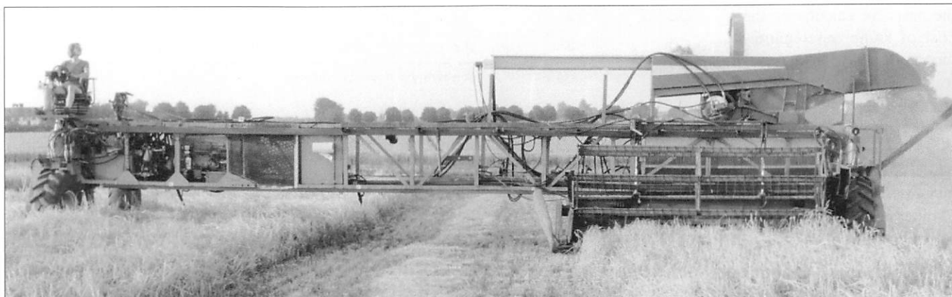
Fig.1 Experimental 75 kW, 12 m span gantry tractor with cereal harvesting unit based on a 4 m moveable header and threshing system.
