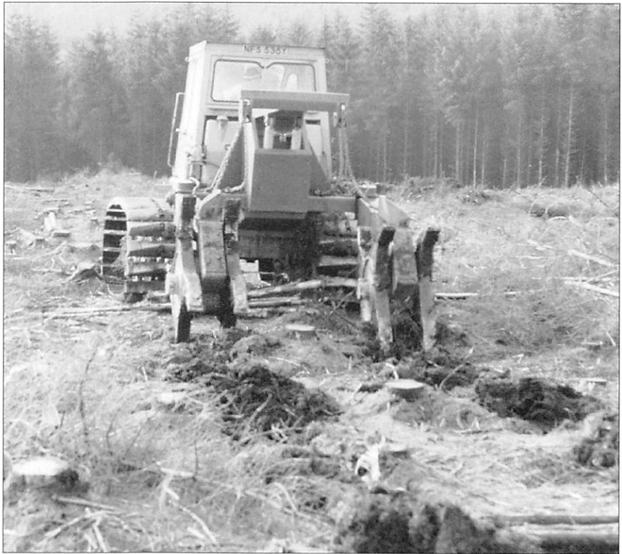
Fig. 1 Caterpillar D6 with Mattock cultivator prepares brash covered land for planting.
