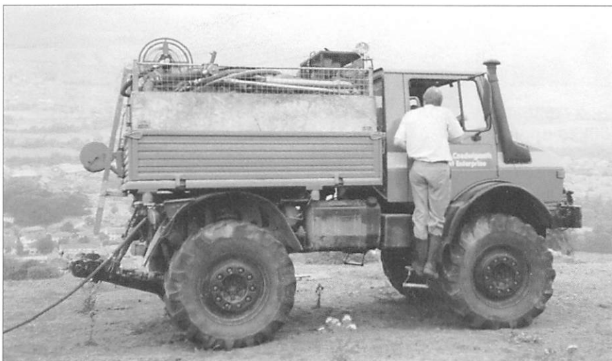
Fig.3 Unimog with a demountable water tank used for fire-fighting duties in Morgannwg, Wales.
