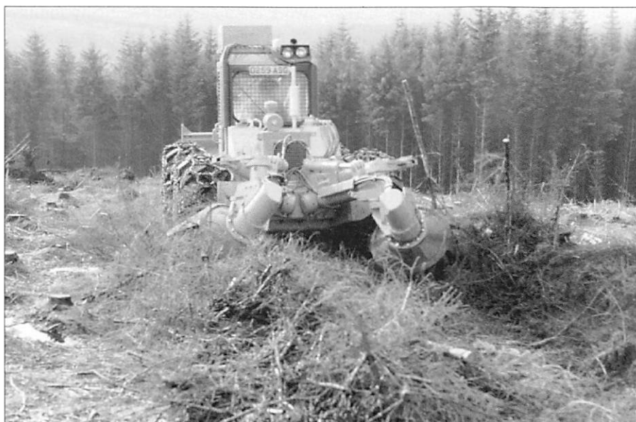
Fig. 2 Timberjack 380A with disc cultivator powered by a Perkins donkey engine.
