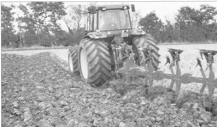
Fig. 1 Large single tyres enable lower inflation pressures down to 0.7 bar to be used when ploughing but are also within the legal limit for road work.
