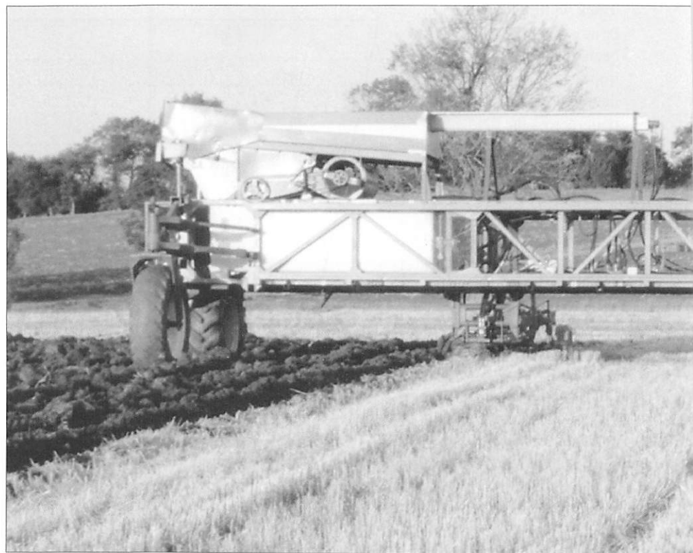
Fig. 3 A 75 kW, 12 m span gantry ploughing to 200 mm depth on a 60% clay soil using two 2 furrow ploughs with opposite handed mouldboards. A 75 kW four wheel drive tractor on conventionally trafficked plots could only pull 3 identical furrows.
