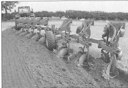
Euromat 3S Herkules 1000 semi-mounted plough comes in six to nine furrow sizes for tractors up to 180 kW.
