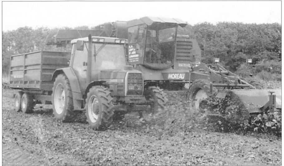
Fig. 2 Trailer based weighing system alongside the sugar beet harvester.
