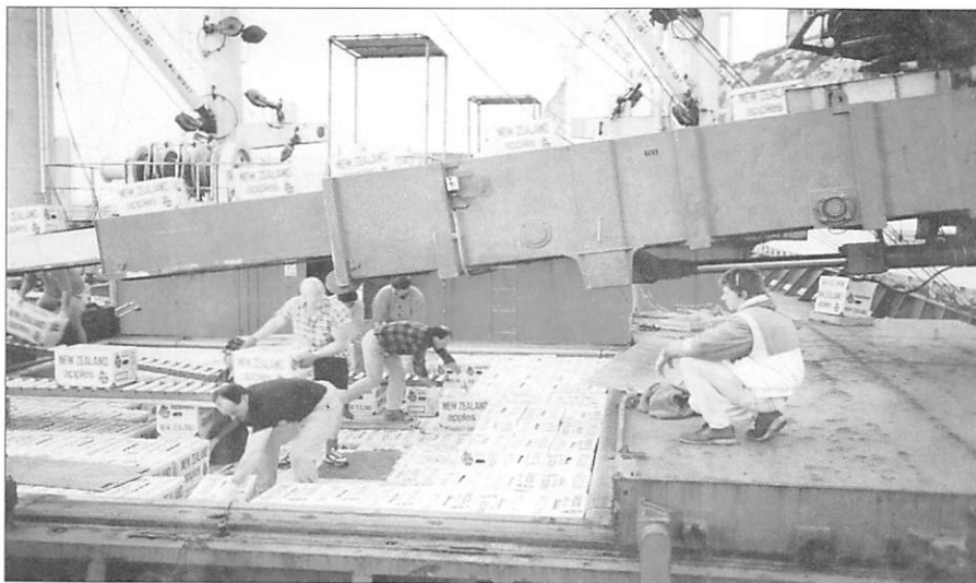
Handling cartons of apples in a ship's hold: note foot boards to avoid bruise damage.
