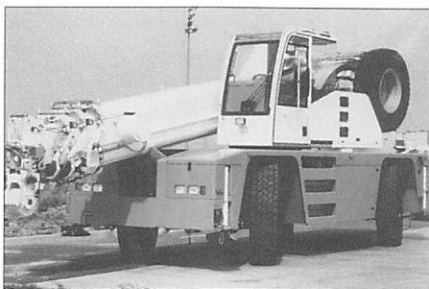
Demag's AC75 City Class crane powered by a six litre Perkins Phaser engine.
