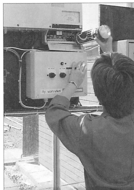
Fig.1 Calibration of an Infra-red Gas Analyser (IRGA) monitoring greenhouse carbon dioxide levels and interrogated by computer controller.
