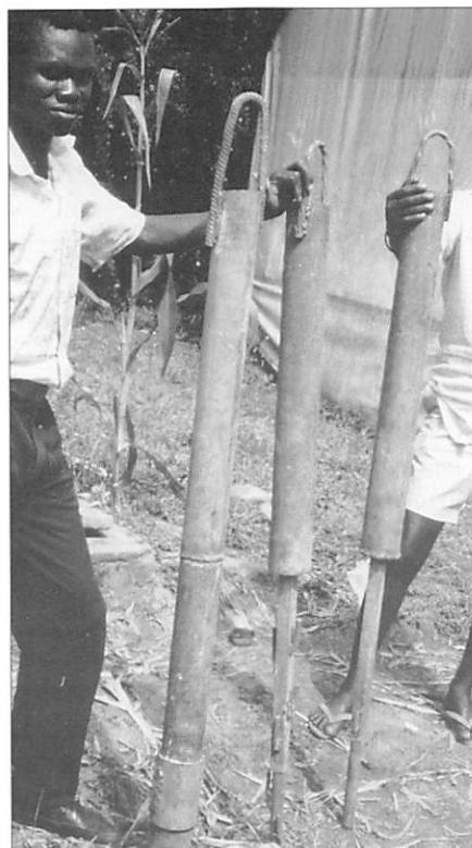
Fig. 3 Some specially made tools: (a) lifter for dropped pipes, both 1 1/4 and 2 1/2 inch (32 and 64 mm); and (b) from L to R, bailer, simple fishing tool, and hammer/prodder.
