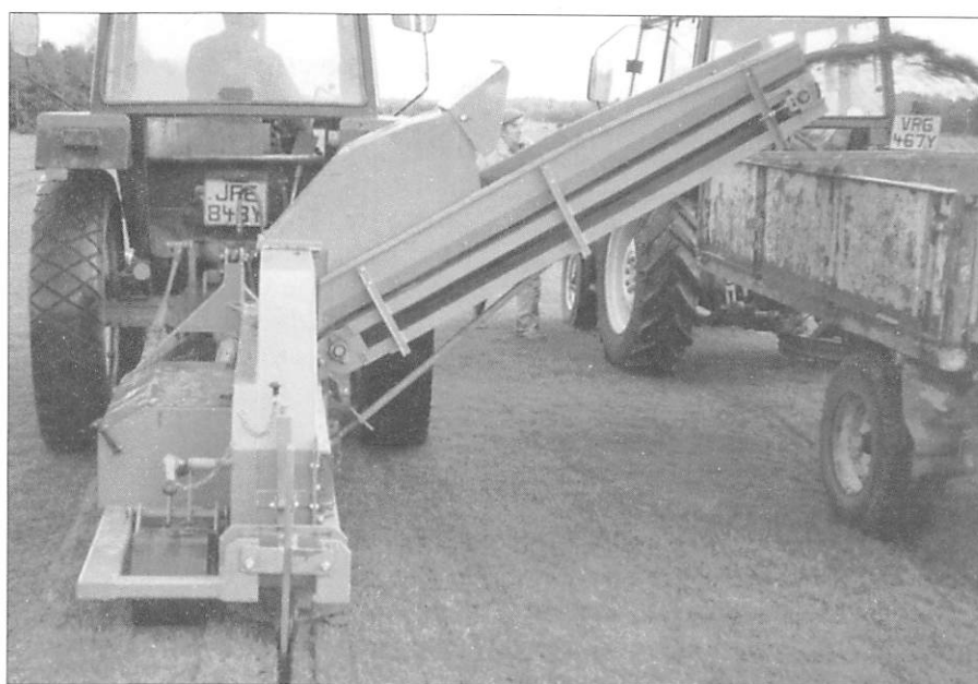
Sand slitting equipment for drainage into existing turf.
