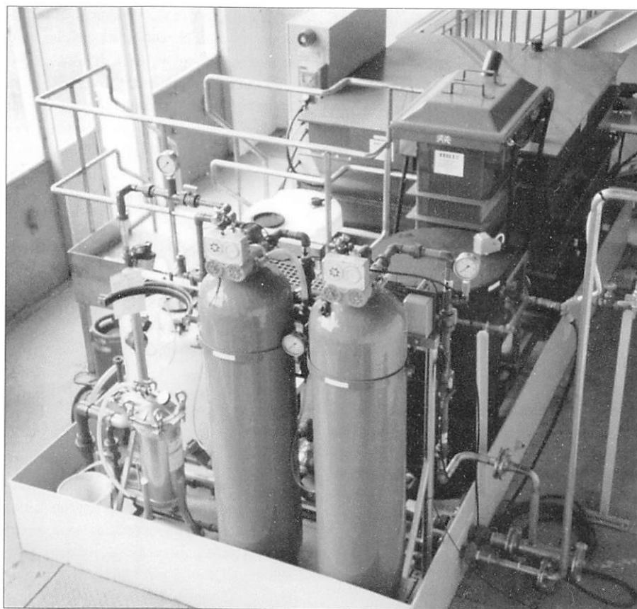
The copper removal plant with the two ion exchange columns (foreground), and the electro-chemical cell and tank in the background
