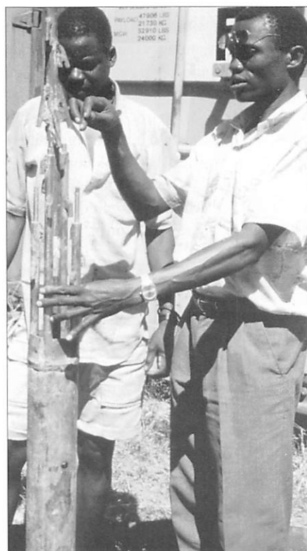
Fig. 3 Some specially made tools: (a) lifter for dropped pipes, both 1 1/4 and 2 1/2 inch (32 and 64 mm); and (b) from L to R, bailer, simple fishing tool, and hammer/prodder.
