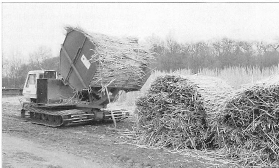
Fig. 3 Making bundles with a reed harvester.
