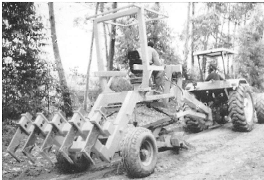
The Simba road grader.....has the potential to provide cost-effective maintenance of unsurfaced roads.
