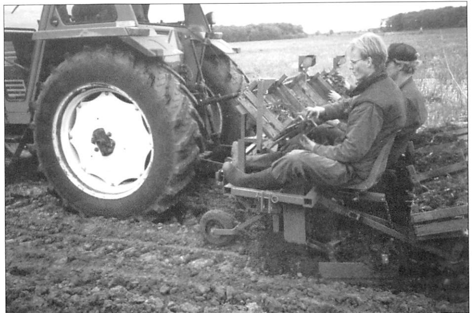
Fig. 1 Planting rhizomes with a specially designed planter.
