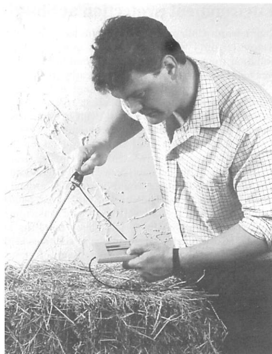
Above: Grainmaster for moisture in grain; Left: Balemaster for moisture in hay and straw bales.
