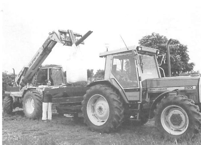
Fertiliser application will be targeted to yield potential with this combination of MF 3120 tractor and spreader controlled by the MF 'Global Positioning System'.
