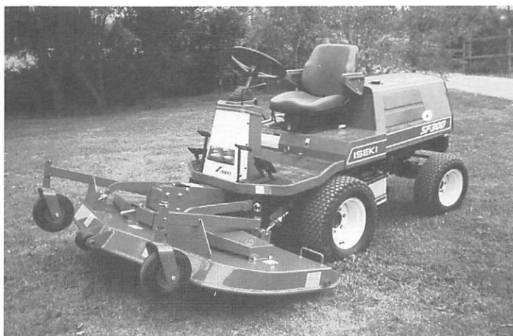
Rotary deck designed for Iseki SF 300.
