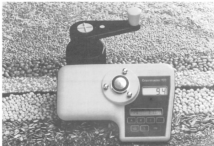
Above: Grainmaster for moisture in grain; Left: Balemaster for moisture in hay and straw bales.
