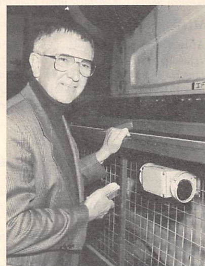
John Boydell inspecting the safety device on a Sedgwick 100-tonne brake press. The device forces the operator to use both hands to operate.
