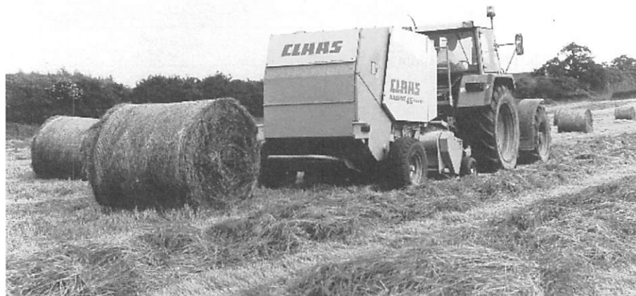
The Claas Rollant round baler with Rollatex net wrapping facility.
