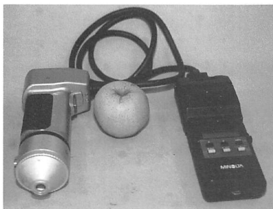
Fig 2. Minolta colour difference meter for measuring change in skin colour during ripening
