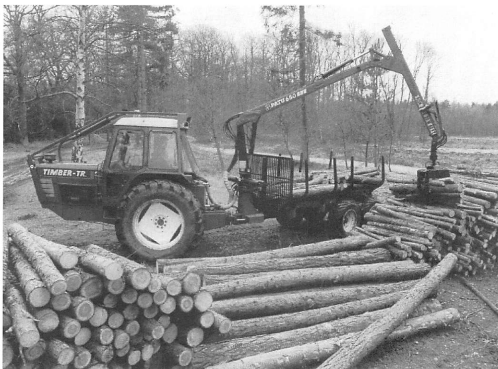
The Caledonian Timber-Trak carries up to 10 t of timber loaded by a 6.5m reach Patu crane.
