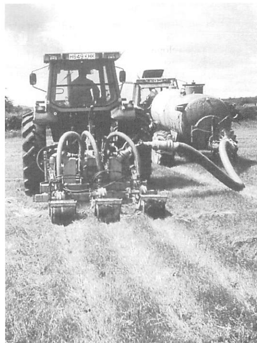
Fig 2. Straight-legged winged injector (WIN) working in grassland.
