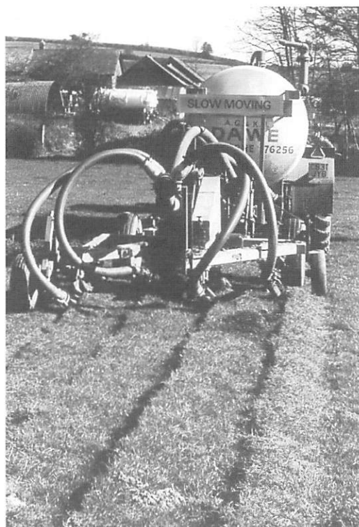
Fig 1. Slant-legged injector (SLA) working in grassland.
