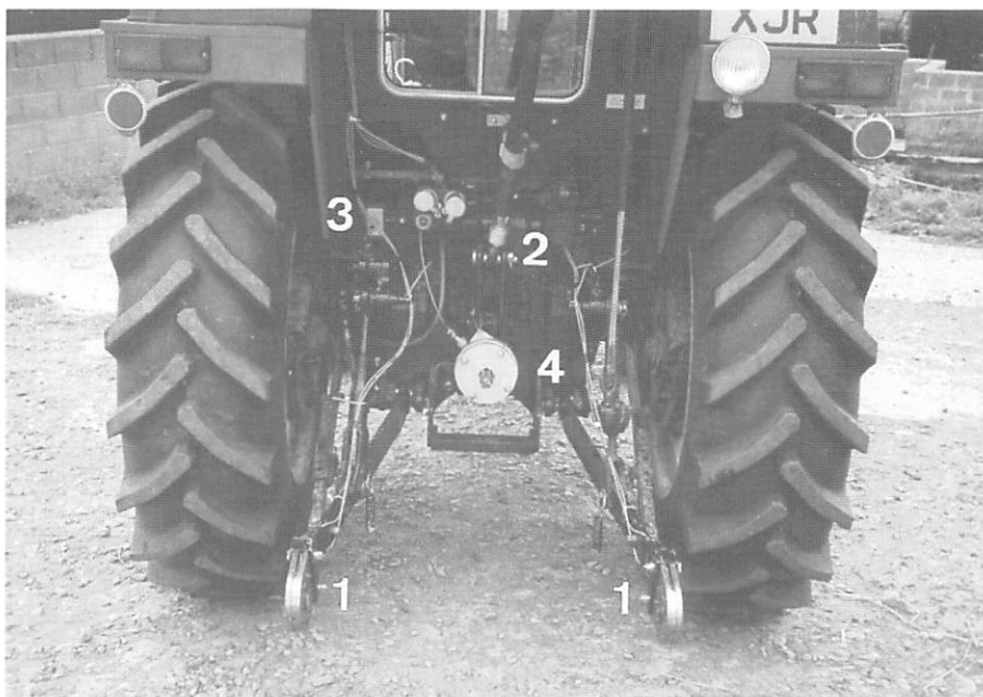
Fig 3. The test tractor – 1) the bottom link transducers; 2) the topline transducer; 3) the linkage position sensor; 4) the torque meter.
