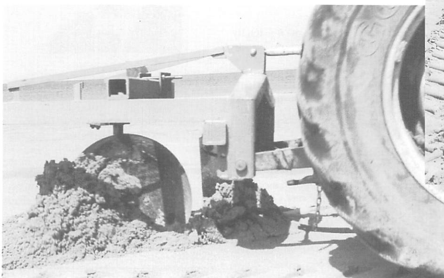
Fig 1. Initial trials using a single unit with serrated and plain discs on Cresswell Beach, Northumberland. a) the tine and disc combination; b) the furrow.
