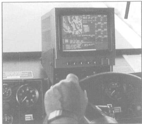
Soilection monitor displays map/field information and status/alert bulletins – all on the same screen.
