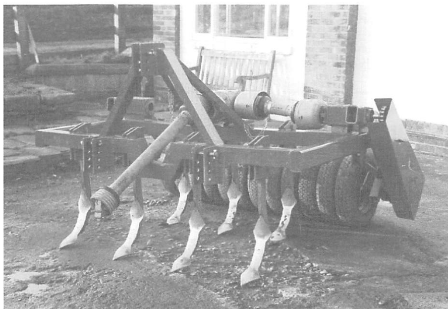
Fig 1. Final design of cultivator; illustrating power transmission line.
