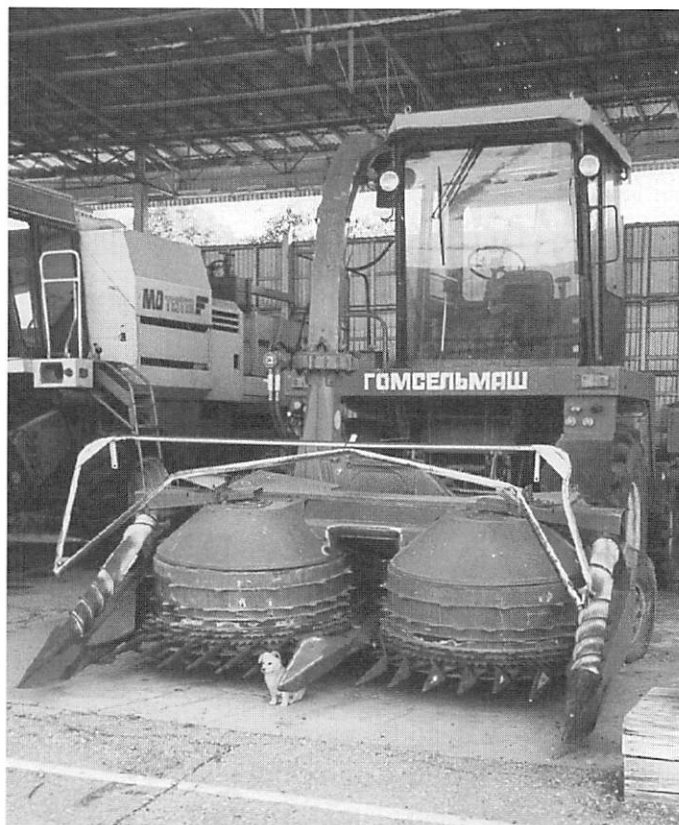
Fig 1A. The changing requirement: This Bulgarian-made maize forage harvester is typical of the large scale machines needed for State farms and large co-operatives. (Contrast this with the small tractor shown opposite).
