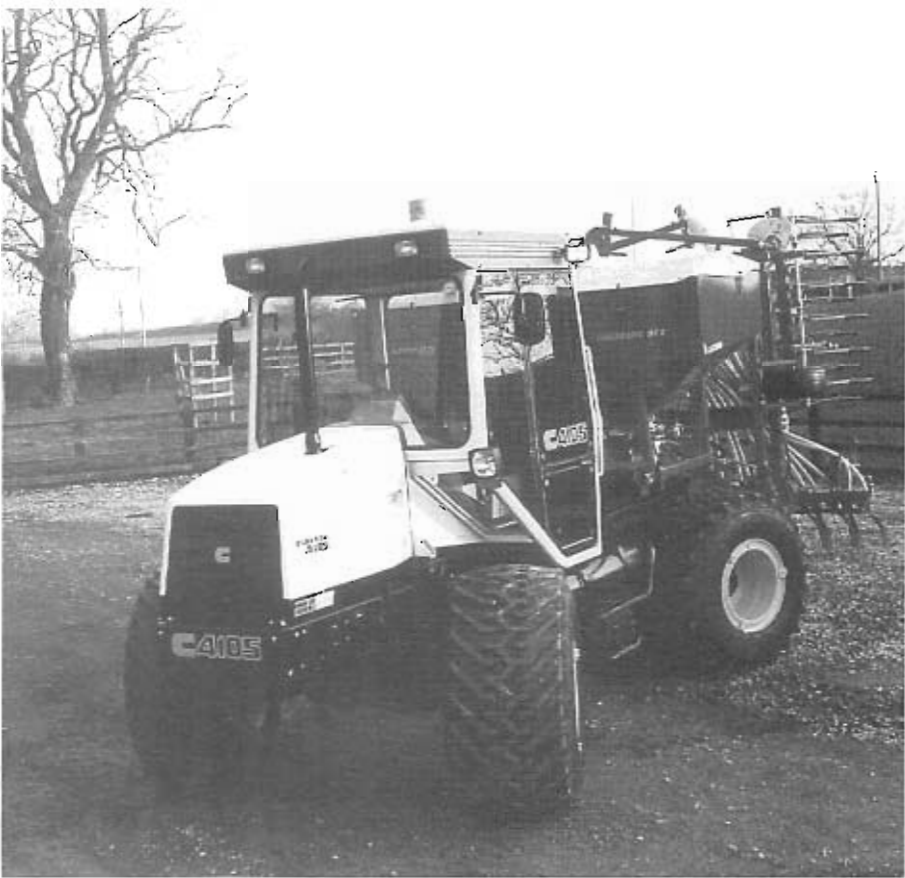
The Clayton 4105 lightweight tractor featuring an air conditioning system designed by Diavia UK.
