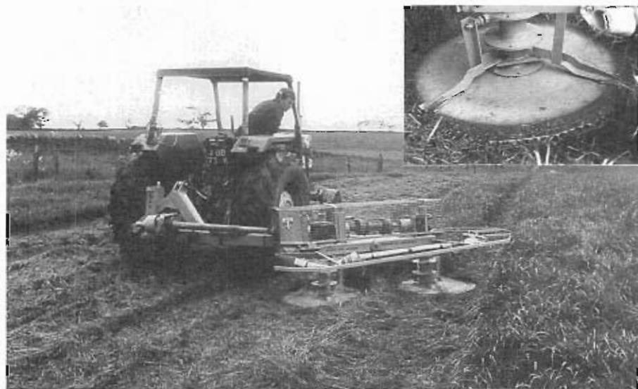
Fig 1. Prototype mower (inset: one of the rotating disc assemblies).
