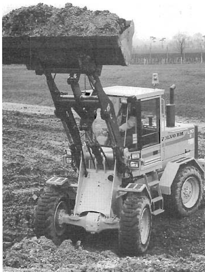
The power behind the Volvo BM L50B shared loader is Perkins' latest low emissions 1,000 Series engine.
