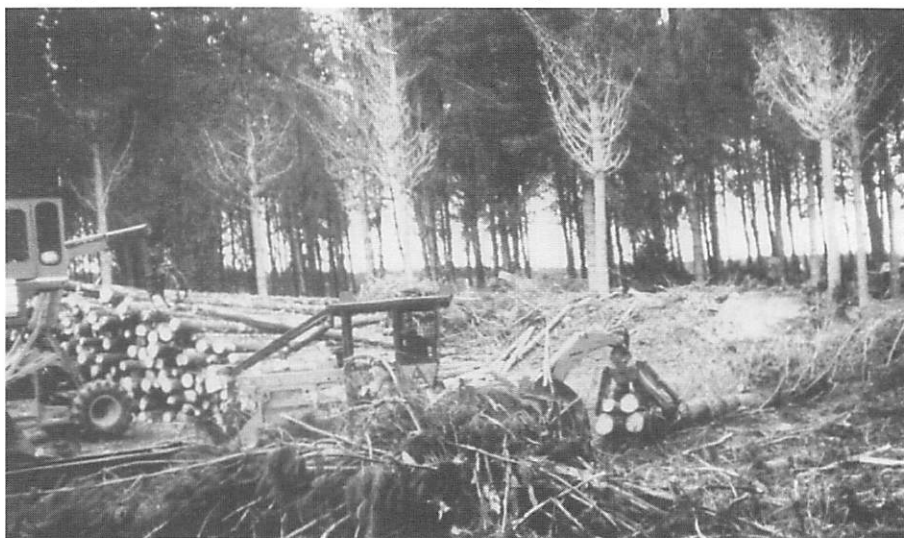
Fig 1. Integrated harvesting of whole Pinus radiata trees whereby processing is carried out at the landing leaving large volumes of residues available as fuelwood.
