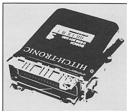
Fig 2a (above). The 'brain' of the system – the Electronic Control Unit.
