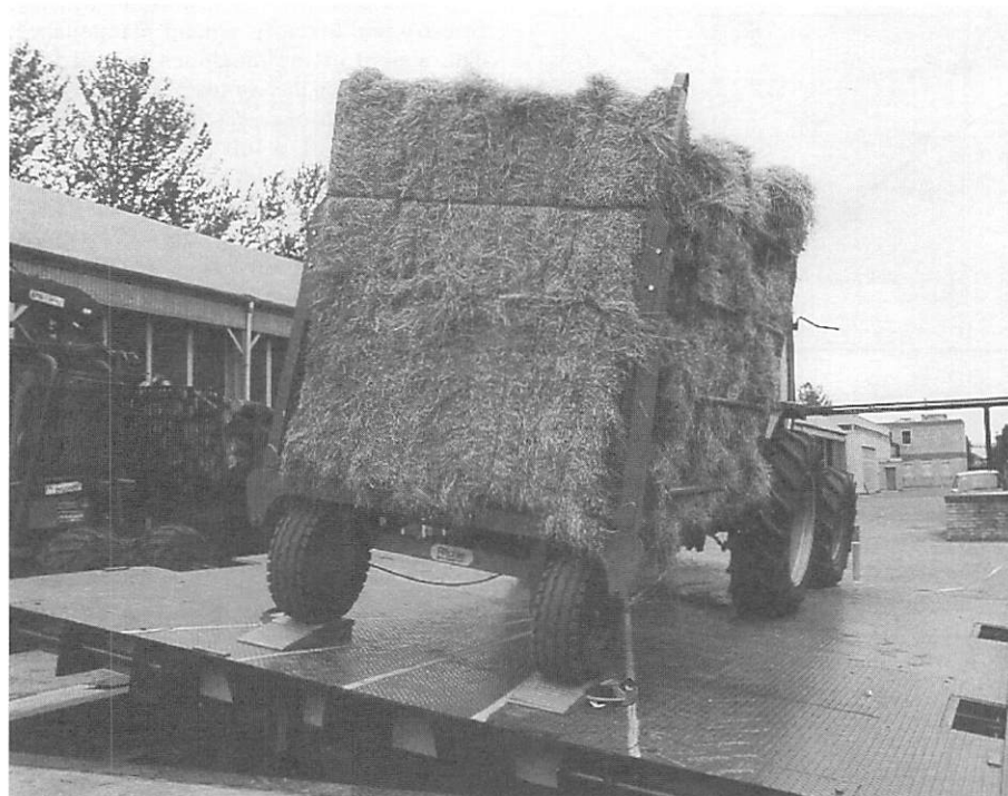
Fig 3. A bale transporter stability test using weighpads on the tilt table.
