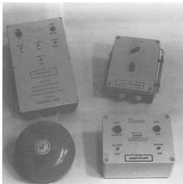
Fig 2. Components of a simple alarm system for livestock housing – control box; bell; high and low temperature thermostat; mains failure unit.
