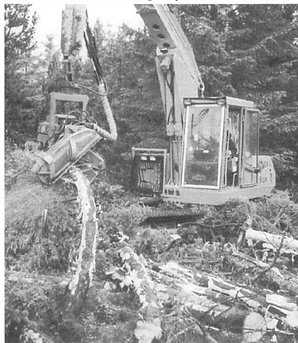
Fig 2. Lako 60 grapple harvester in lodgepole pine.
