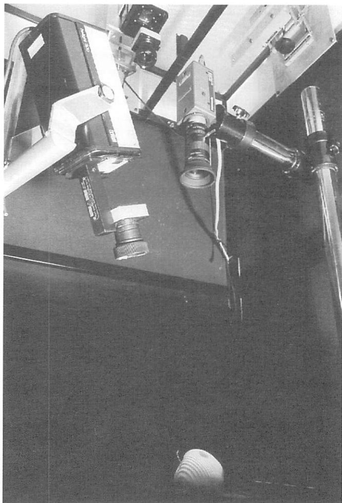
Fig 2. Blemish detection for automatic apple grading – structured light can be used to detect the stalk and calyx areas of an apple. (Photo: Silsoe Research Institute.)
