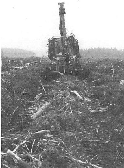
Fig 1. A thoroughly sound brash mat is essential for soft ground harvesting operations.
