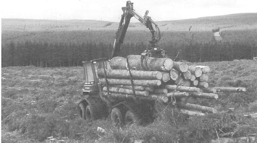
Fig 3. Band tracks are usually essential for soft ground working.
