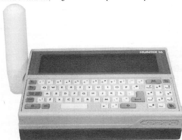
Fig 3. The Navstar XR4, a Husky portable computer fitted with a GPS receiver.
